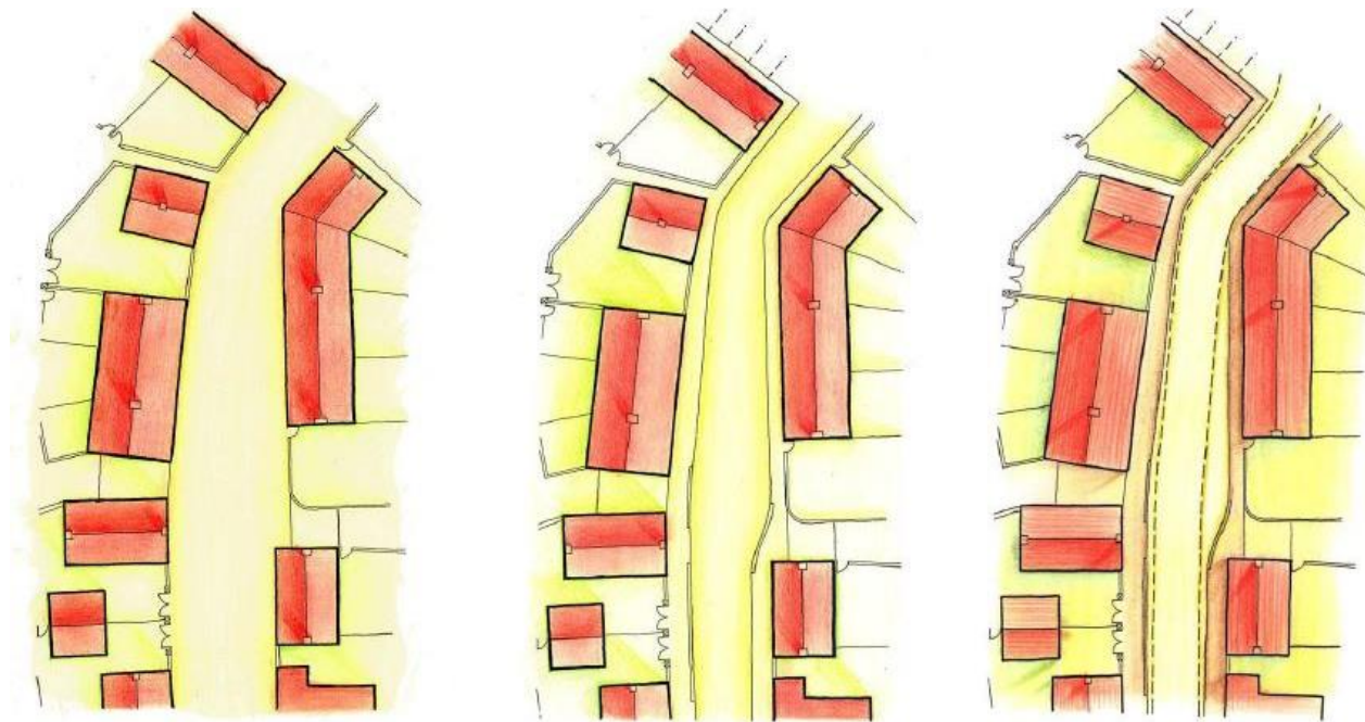
Figure 5-4: The built form should determine the carriageway design (Credit – Manual for Streets)
