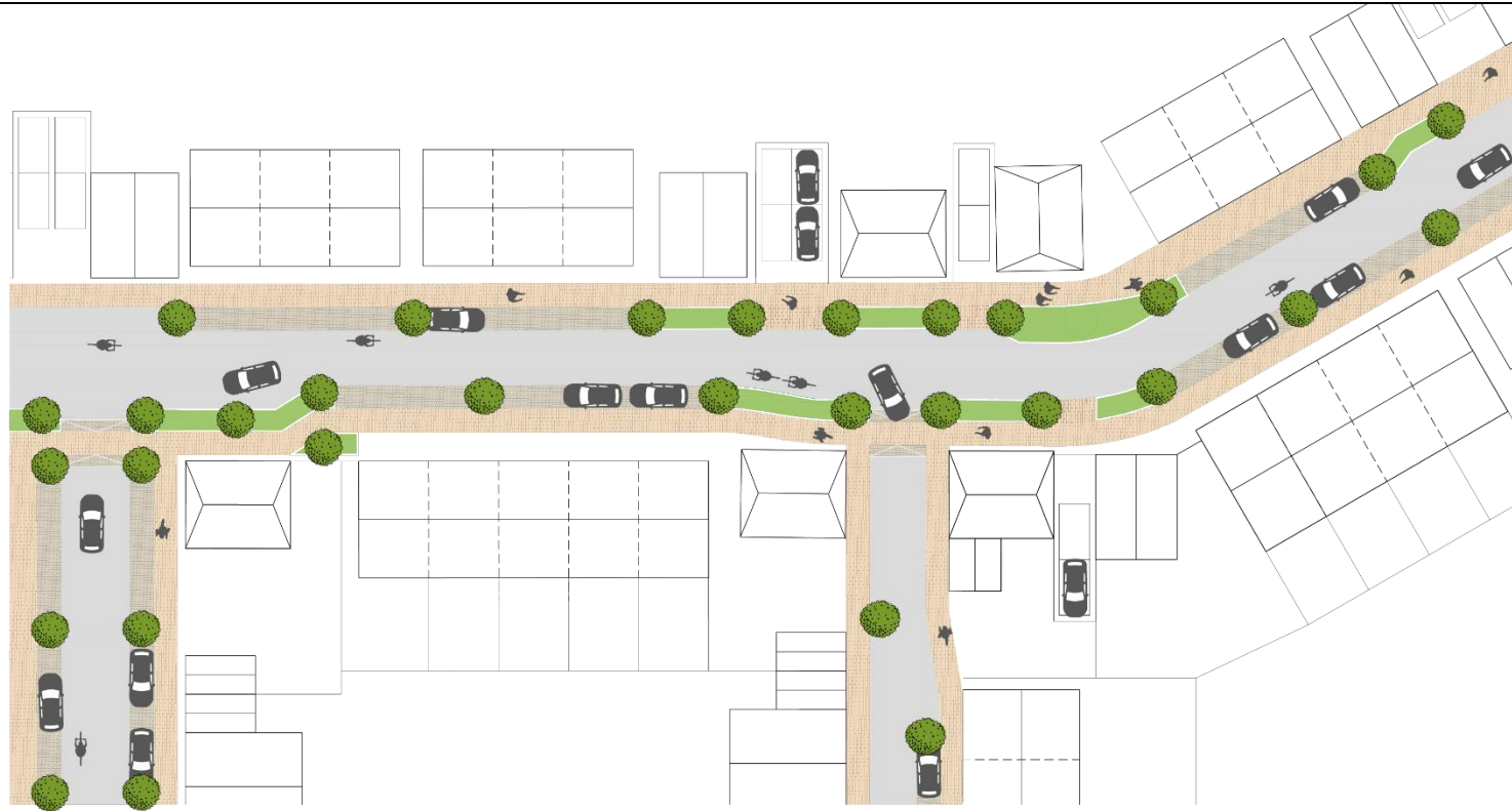
Figure 4-17: Typical Layout Diagram – Type 3 – Secondary streets
